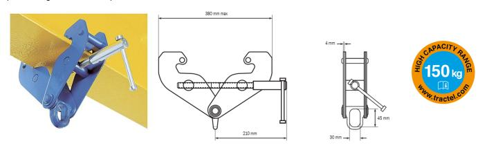
The Corso clamp anchoring device is intended exclusively for the docking of a personal protection system against falling heights, for example an energy absorbing lanyard or automatic fall arrester blocforTM or rope grabs stopfor <sup>™</sup>. The Corso clamp can be installed on the bottom flange of an I, H or T beam.
